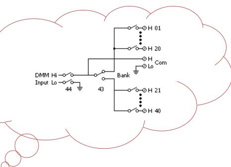
DAQ-903 can switch 40 single-wire inputs per module. It can be used for common-low applications such as battery testing, component characterization and desktop testing. The low-voltage connection is isolated from ground and can be floated up to 300 V.
