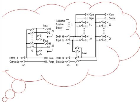
DAQ-901 is a comprehensive multiplexer for general scanning. The same module can mix 2-wire and 4-wire channels; at the same time, the additional 2 current input channels can be used for AC and DC current measurement without external shunt resistors (maximum 1 A per channel).
