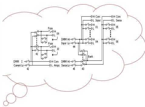
DAQ-909 is a multiplexer specially designed for high voltage, providing 8 channels for DC 600 V / AC 400 Vrms voltage measurement. The additional 2 current input channels can be used for AC and DC current measurement, external shunt resistors are not required (maximum 2 A / per channel).
