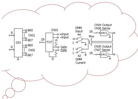
DAQ-907 provides great flexibility for various sense and control applications. It engages two 8-bit digital input and output ports, a 100 kHz gated totalizer, and two  $\pm$  12 V or  $\pm$  24 mA analog outputs—all on a single earth-referenced module. The digital inputs and totalizer input may be included in a scan. Alarm limits for the digital and totalizer inputs are evaluated continuously, capturing and logging alarm conditions even between scans.
