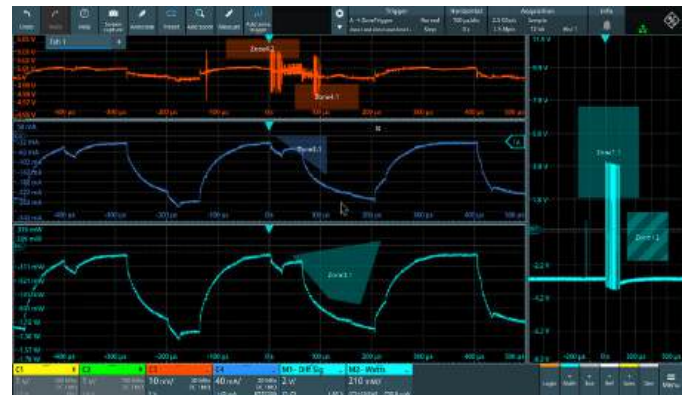
Power rail measurements with zone trigger to isolate power consumption events during RF transmissions
